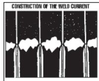
*Subsequent melting and the formation of new bridges allow the weld to be formed.*
