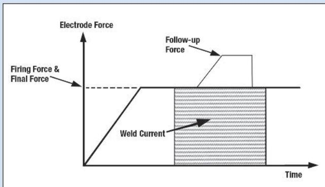
Recent advances in weld head design include electronic weld heads where weld head movement and force are electronically controlled, and/or electronically monitored, via a precise schedule. The precise control of an electronic weld head can program the timing of each element of the force profile, minimize impact force, duplicate force profile between weld stations, and provide electronic evidence of the actual
