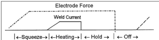
This basic weld schedule forms the basis for all microwelding schedules. The amplitude and duration of all force and heating parameters can be defined in the “weld schedule.” The four critical parameters are: electrode force, squeeze time, weld pulse and hold time. Variations can also be dual pulse and other sequences shown below.
