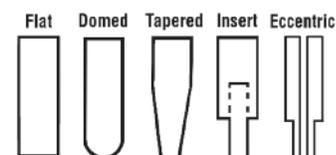
The size of the weld will not be larger than the electrode face. Therefore, it is important to utilize electrodes of the same tip diameter as the desired weld nugget. The current density at the workpiece interfaces varies as the square of the diameter of the electrode face. Electrode positioning is critical: electrodes
