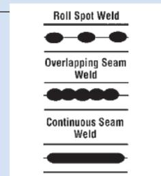
**Seam Welding** is another variation on resistance spot welding. In this case, the welding electrodes are motor-driven wheels rather than stationary rods. The result is a "rolling" resistance weld or seam weld used to join two sheets together. Overlapping and continuous seam welds can produce gas- or liquid- tight joints.
