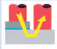
**Step (Indirect) Welding** is often used when the workpieces are configured in such a way that only one side of the workpiece is accessible with an electrode, or there is a large thermal imbalance. The welding current flows from the first electrode, through the workpiece, through the area of the weld, through the other workpiece and into the other electrode.
