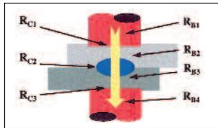
**CONTACT RESISTANCE** is a function of the extent to which two surfaces mate intimately or come in contact. Contact resistance is an important factor in the first few milliseconds of a weld.
