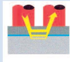
**Series Welding** is also used when only one side of the weldment is accessible with electrodes. This form of welding has the advantage of making two weld nuggets at one time. However, series welding is generally less controllable because of the many shunt paths available to the welding current.
