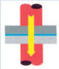
**Opposed (Direct) Welding** is the most commonly used type of resistance welding. The welding current flows directly from one electrode to the other, through the weldments.
