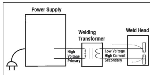
In simple terms the resistance welding power supply transforms, modulates and controls the electrical energy of the power line and applies it to the weld according to a user defined or user programmed “weld schedule.” Depending on the complexity and intricacy of the power supply the user can program from one to more than 100 attributes and permutations of the welding process, and, using a microprocessor, store these attributes as a uniquely defined “weld schedule.”
