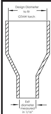
Most nozzles used for GTAW are manufactured from ceramic materials, alumina (pink colored) and lava (white colored). The exit diameter (diameter closest to the arc) is manufactured in a variety of sizes, GTAW nozzles are also made in various lengths from short nozzles to extra-long nozzles.
