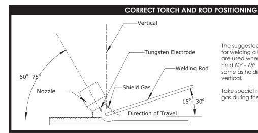
The suggested electrode and welding rod angles for welding a bead on plate. The same angles are used when making a butt weld. The torch is held 60° - 75° from the metal surface. This is the same as holding the torch 15° - 30° from the vertical.
