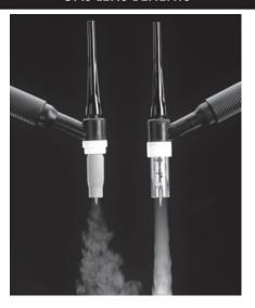
A collet body with a gas lens can be very useful to a welder. The purpose of a gas lens is to make the shielding gas exit the nozzle as a column instead of as a turbulent stream of gas that begins to spread out after exiting. The column of gas allows the electrode to stick out farther for visibility, allowing for better access to the weld area, and a reduction in gas flow (CFH/L/Min).
