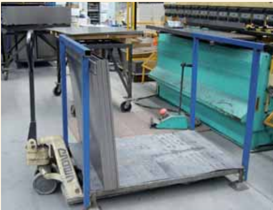
Pallet jacks assist in movement of product throughout the shop floor.
