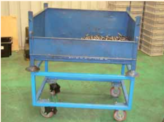
This stillage has been raised so it is between knee and shoulder height.
