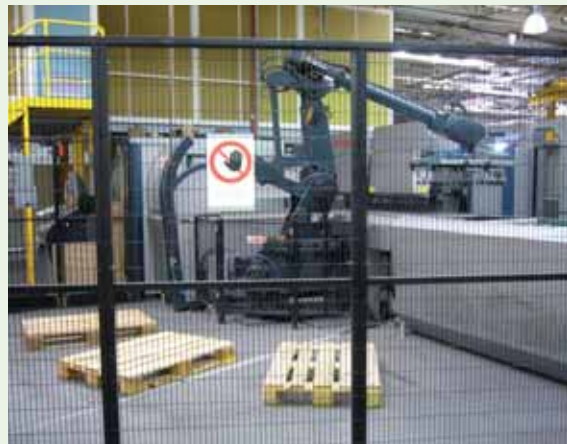
This robot takes punched sheet metal and stacks it onto a pallet.
