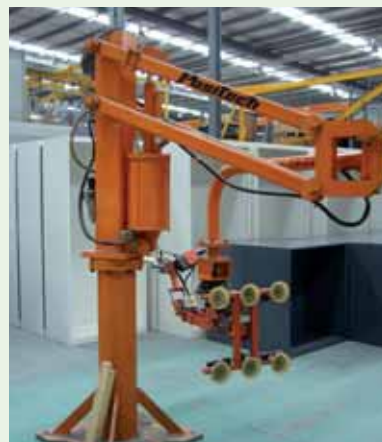
A manipulator is used to transport product to another workstation.
