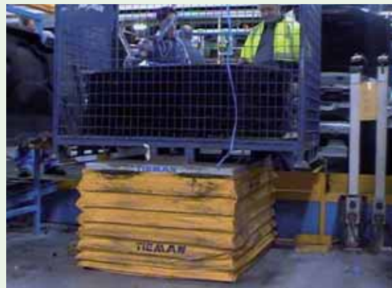
This stillage with drop down sides is on a scissor lift to raise the product to a good working height.
