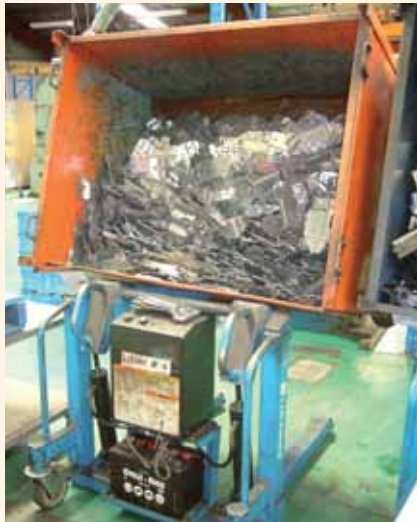
This stillage is tilted for easier access.
